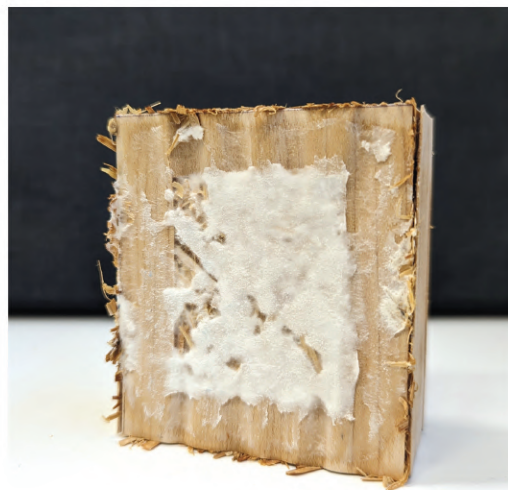
Mycelium - veneer composite
